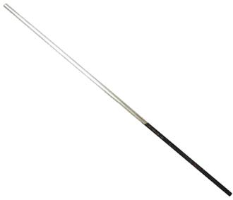
This unit is equipped with a metal Media Bed Indicator. The indicator is positioned inside the system at an angle against the direction of airflow and detects the expiration level of the media.
