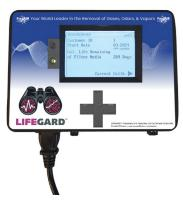
Equipped with externally wired and mounted sensors, the media bed monitor detects variations in adsorbent media life with precision. These sensors relay data to the controller, which uses a proprietary algorithm to accurately forecast the media consumption date, streamlining maintenance scheduling and enhancing efficiency.
